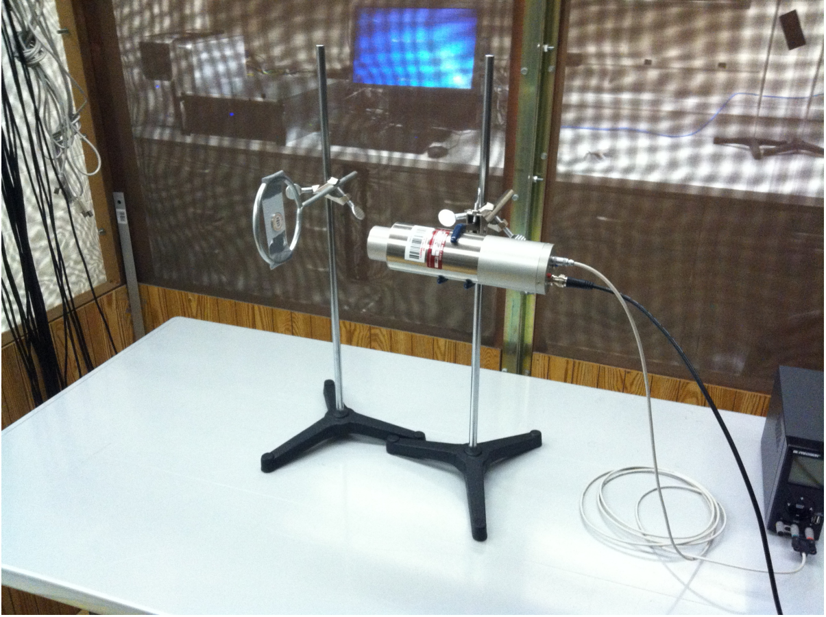
Figure B.2: \text{CeBr}_3 with calibration source setup to collect PHS to validate fitting algorithms PHS.
